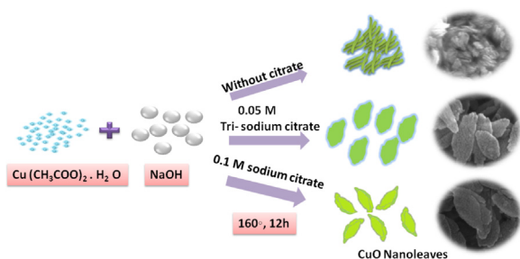
Fig. 4. Schematic illustration of formation of CuO nanoleaves.
